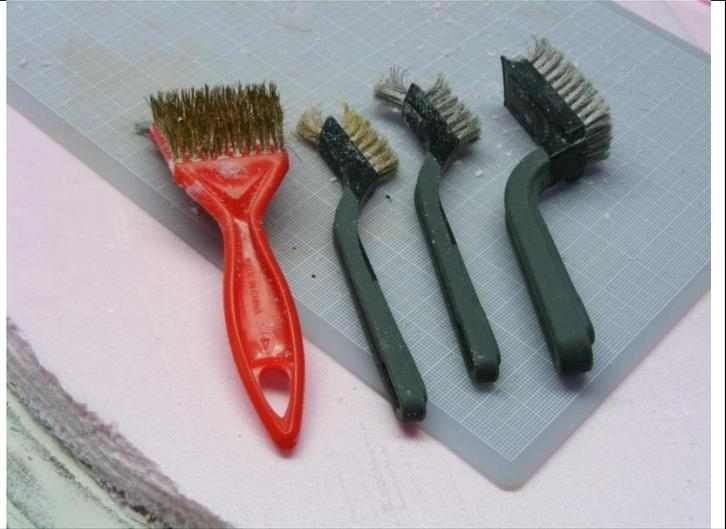
3. Wire brushes are used to take the foam board that has been cut to the final stage of developed scenery. Wire brushes are good for howling out indentations, creating exposed rock on the sides of cuttings, smoothing the tops of hills and creating fields, streams and rivers. Brushes are made
