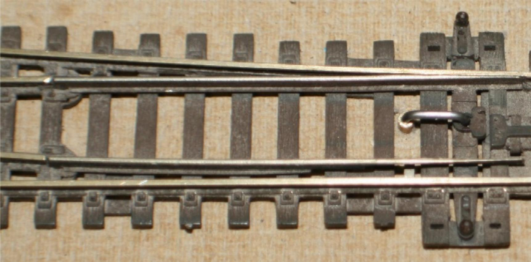
Many people bring music wire above the ties to connect to the throw bar. I find this objectionable. 0.047" music wire is over 4 inches in HO scale 0.055" is 4-3/4". Way out of scale to be on top of the track. I designed a way to bring the actuator wire from underneath to minimize its appearance. See the instructions for building the base.
