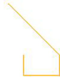
Brass strip after bend (edge view)
